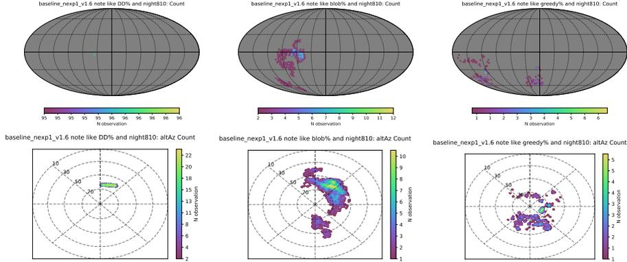
**Figure 4.** Examples of how the three scheduler tiers execute during a single night. Left panels show how a DDF sequence was observed during the night. Middle panels show observations taken as part of blob pairs. Right panels show the greedy observations taken in twilight time. The panels from left to right show the different decision tiers the scheduler uses, with the DDFs as the top tier and the greedy algorithm as the bottom tier.
